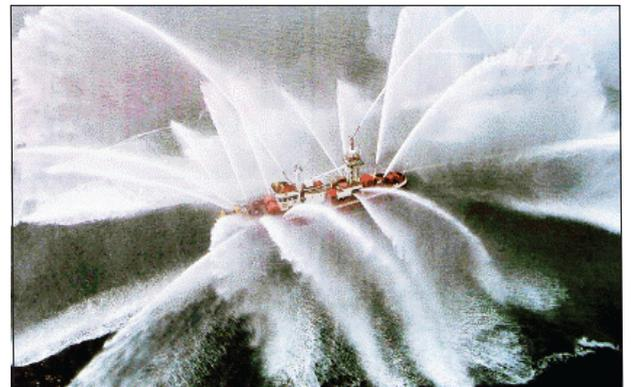
Multiple water cannons aboard LAFD Fireboat 2 can deliver a stream of water over 400 feet (120 m) at a rate of 38,000 gpm (143,830 liters/min).
