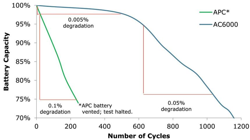
Figure 1. Capacity degradation comparison during full-power discharges at 25°C.
