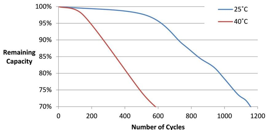
Figure 2. Li-ion UPS at 100% DoD at Ambient and High Temperature.
