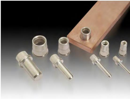
The embedded PowerBud connectors have knurled outer side walls allowing direct press-fit insertion into bus bars, printed circuits boards and FusionLugs™. Installation or press-in is accomplished using any flat surface and does not require any special tooling. The current rating is dependent on the physical size of the pin and the heat-sinking capability of the mounting medium.
